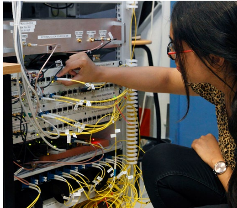
Illustration : An experimental 500 km White Rabbit link in the testing phase at the Observatory of Paris. Credits : Pascal Blondé, LNE-SYRTE, Observatoire de Paris
